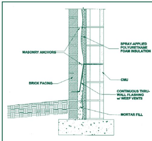
**Figure 6: Detail of through-wall flashing and footer.**
