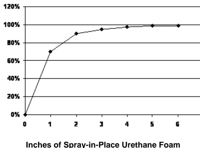
*This graph illustrates the reduction in heat loss from a building when it is insulated with various thicknesses of spray-in-place urethane foam. Note: the insulation benefit tops off very quickly above three inches. The graph is*
