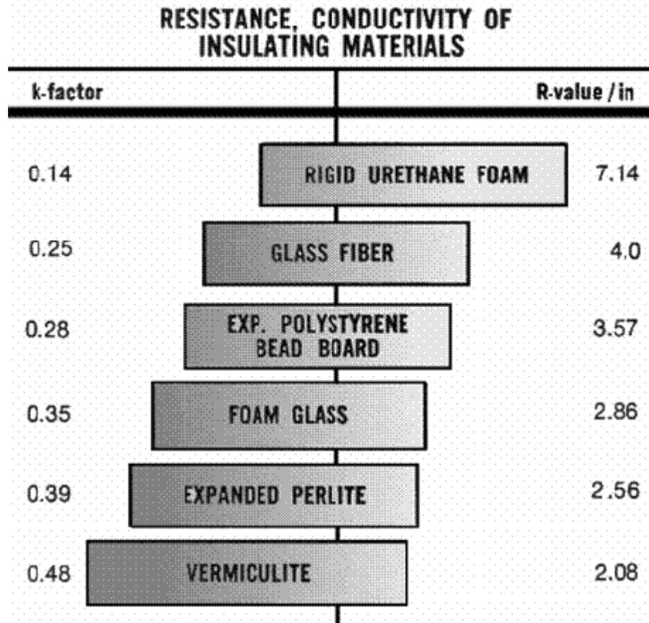
*With the lowest k-factor and the highest R-value, urethane foam can provide more thermal resistance with less material than any other insulation.*
