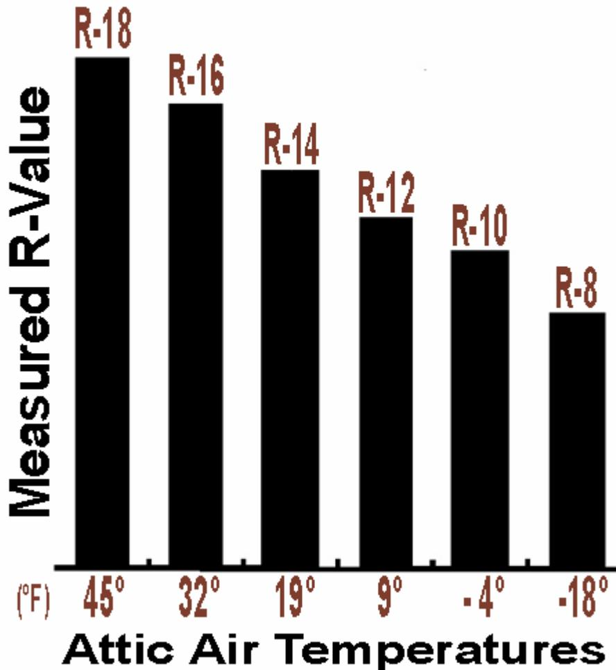
*In full-scale attic tests at Oak Ridge national Laboratory, the R-value of 6 inches of cubed loose-fill attic insulation progressively fell as the attic air temperature dropped. At -18° F, the R-value measured only R-9. The problem seems to occur with any low-density, loose-fill fibrous insulation.*
