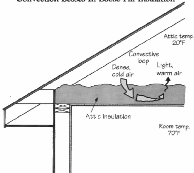
*At very cold temperatures, when the temperature difference across the attic insulation reaches a certain critical point, convection within the insulation can reduce R-value.*
