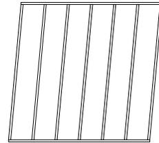
Stud wall under shear load (exaggerated)
